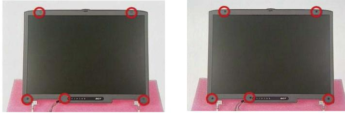
6. Snap off the bezel carefully, and then remove the LCD bezel from the LCD module.
