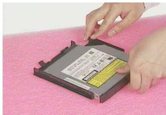
5. Remove the two screws and then detach the optical drive PCB from the optical drive module.
