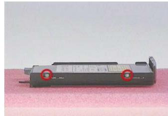
4. Detach the optical drive module from the optical drive chassis.
