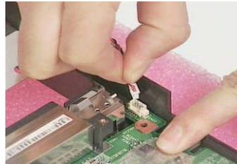
14. Remove the three screws as shown and detach the main board from the lower case carefully in the way as shown here.
