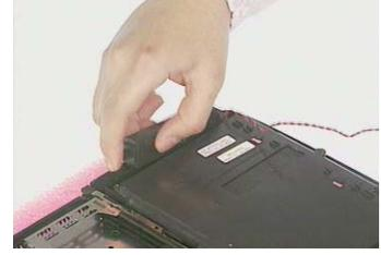
**NOTE:** Please pay attention to how the speaker cable is routed when the speakers are attached back to the main unit.
