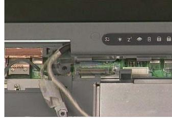
6. Remove the inverter cable from the main board with a plastic flat screwdriver.
