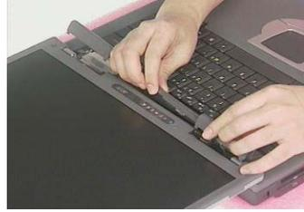
3. Turn the middle cover over and disconnect the launch board cable from the launch board and then detach the middle cover away from the main unit.
