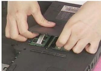
4. Push out the latches on both sides of the socket and pull the memory module out from the socket.
