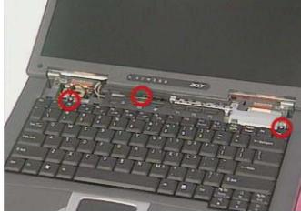
4. Lift the keyboard upward carefully and put it on the upper case.
