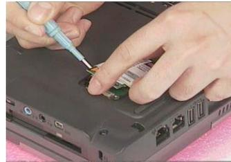
5. Disconnect the modem cable from the modem board, then remove the modem board.
