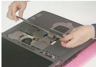
5. Use a plastic flat screwdriver to help disconnect the keyboard cable from the main board carefully, then remove the keyboard from the main board.
