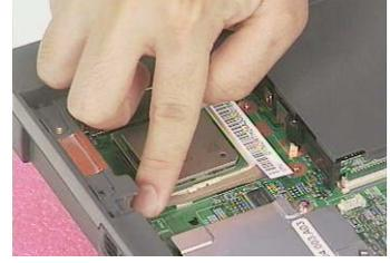
**NOTE:** Please make sure the CPU is attached with PIN1 on this side.
