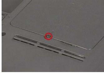
3. Lift the cover off, and then remove the memory cover.
