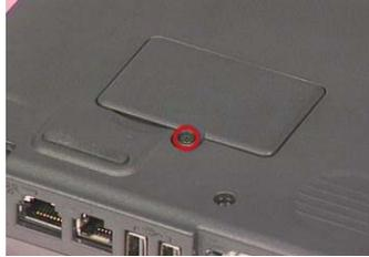
3. Remove the modem cover from the machine.
