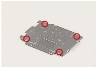
5. Detach the hard disk drive bracket from the hard disk drive.
