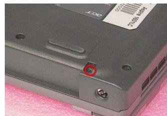
5. Remove the screw and disconnect the LCD coaxial cable from the main board.
