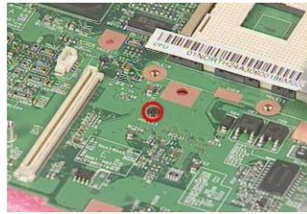
**16.** Detach the I/O port bracket from the main board.
