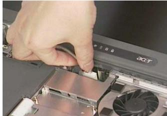
7. Remove the four screws as shown and then detach the LCD module from the main unit carefully.
