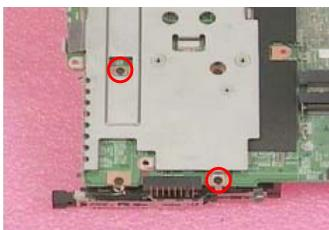
15. Remove the two hex screws and the other one screw as shown to detach the I/O port bracket from the main board.
