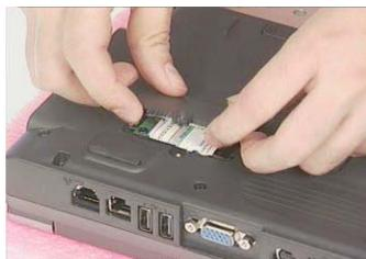
4. Remove two screws from the modem board as shown, disconnect the modem cable from the modem board, and then remove the modem board from the main unit carefully by using a plastic flat bladed screw driver.
