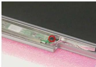
7. Disconnect the LCD power cable, remove the inverter board from the LCD panel, and then disconnect the inverter cable from the inverter board.
