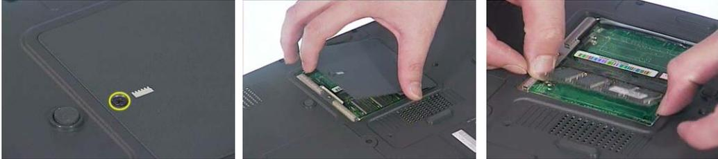
4. Unscrew the two screws that secure the HDD module.
