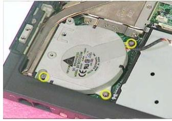
3. Unscrew the five screws that secure the thermal module then remove the thermal module.
