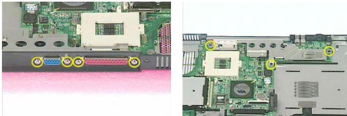
17. Unscrew the four screws that lock the main board.
