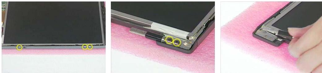
7. Disconnect the inverter board power cable and LCD CCFT cable then remove the inverter board.
