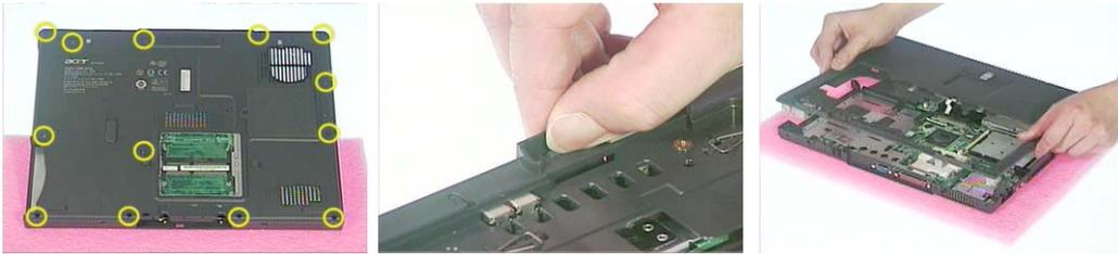
13. Unscrew the four screws that secure the FDD module.
