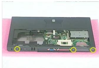
10. Remove the thirteen screws on the base panel.
