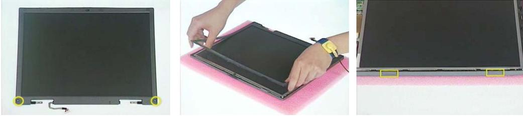
4. Unscrew the six screws that fix LCD to the LCD panel; three on each side.
