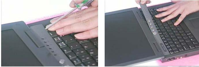
3. Unscrew the three screws that secure the keyboard. Next, turn over the keyboard.
