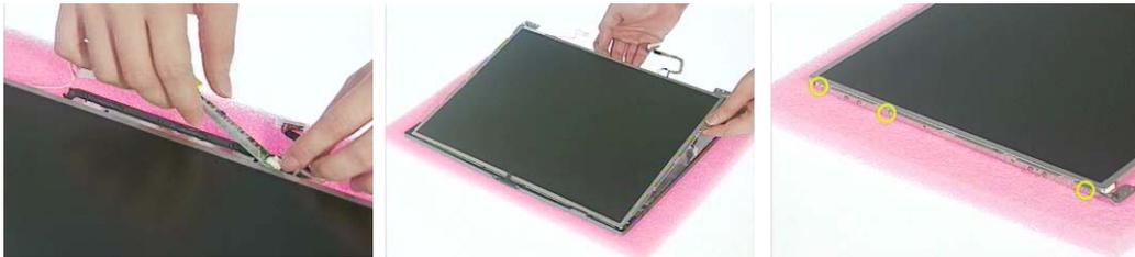
10. Tear off the conductive fabric tape.
