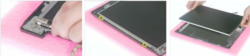
8. Remove the four screws that lock the right and the left LCD brackets. Two on each side.
