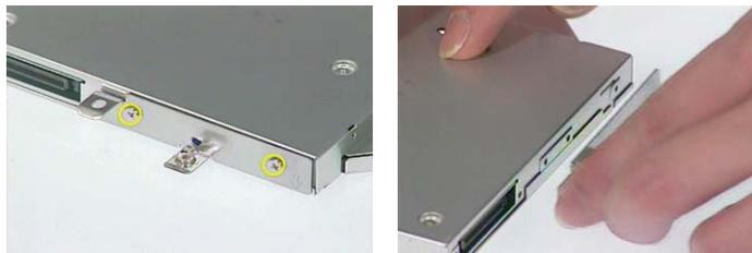
3. Remove the two screws that lock the ODD door.
