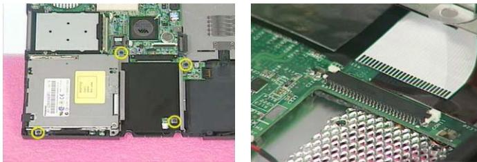
15. Remove the four screw nuts on the rear panel.
