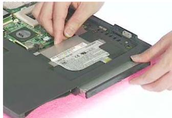
7. To detach the upper cover from the main unit, first disconnect Tear the mylar from logic upper assembly.
