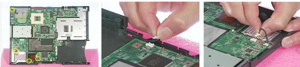
20. Remove the main board off the lower case.
